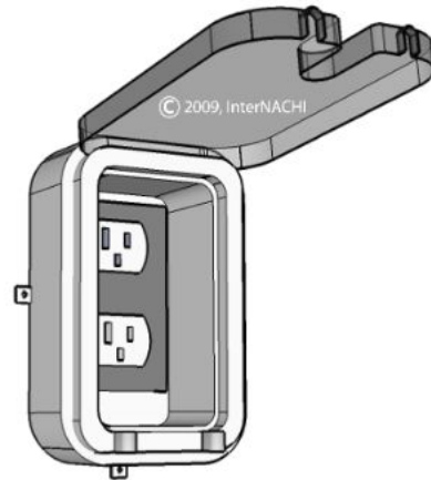
Illustration of proper weatherproof cover plate.
